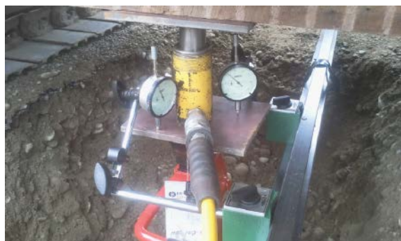
Close up view of dial gauges and hydraulic jack in test 1
