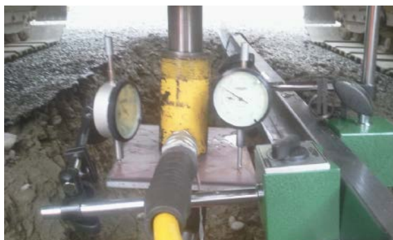
Close up view of dial gauges in test 1
