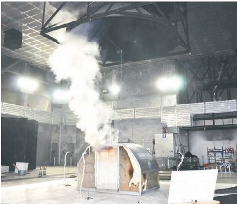
Smoke billows from an aluminum and polycarbonate cargo container during flammability tests.
