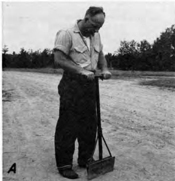
FIGURE 15.—A, A hand trencher for transplanting operations. Blade, 2 pieces of \frac{1}{4} -inch steel 14.5 by 6.5 inches in size, 2-inch spread at top; handle, 32.5 inches long; handle grip, 1-inch iron pipe 13.5 inches long; braces, \frac{1}{2} -inch solid iron bars. B, A tractor-drawn trencher.
