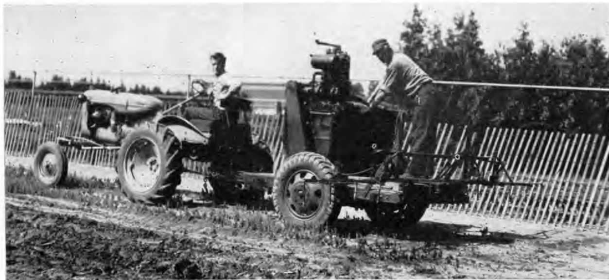
FIGURE 42.—Spray rig for applying mineral spirits.
