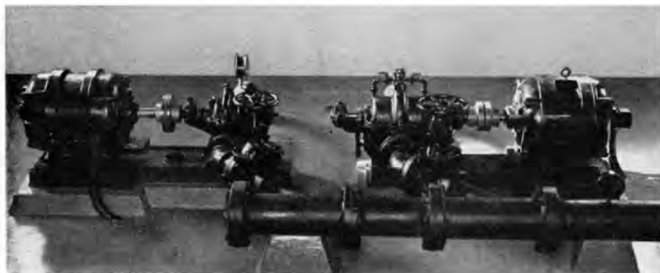
F-313452 FIGURE 8.—Pump on right is a 225-gallon-per-minute, double-suction centrifugal, driven by a 15-hp., single-phase, electric motor. Pump on the left is of the same type and capacity but made by a different manufacturer.
