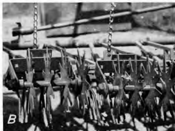
FIGURE 17.—Rotary weeders for seedbeds sown in drills. A, Overall view; B, closeup of rotary hoe units.
