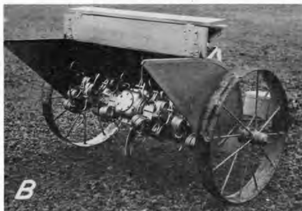
FIGURE 12.—A, A self-propelled rotary tiller. B, A 4-foot rotary tiller operated by power takeoff from a tractor.
