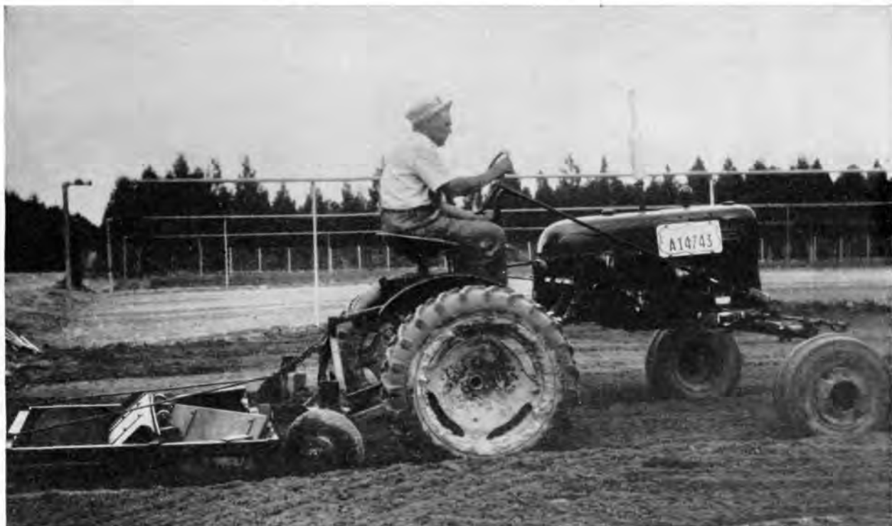
FIGURE 35.—A seedbed shaper of commercial manufacture.
