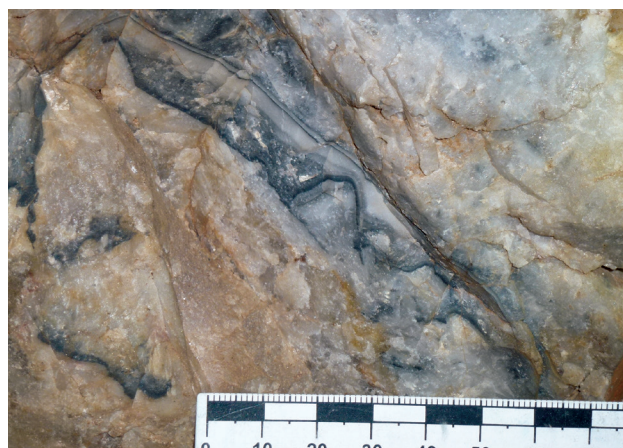
Figure 35. Close-up of quartz breccia vein in the Summit mine, Steeple Rock district. The thin black veins contain gold, silver, and pyrite (NMGR0459). Photo by Virginia T. McLemore.
