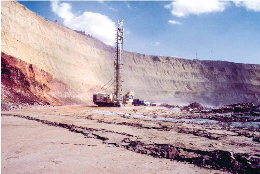
Rig drilling blast holes on a bench at the Tyrone Mine, 1999 (NMGR0084). Photo by Virginia T. McLemore.
