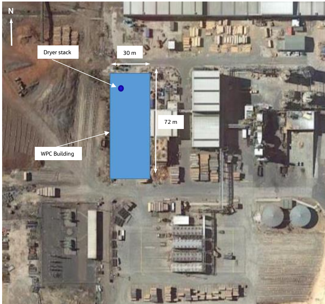
Figure 6-1: Dryer stack location (approximate) on roof of WPC Facility building
