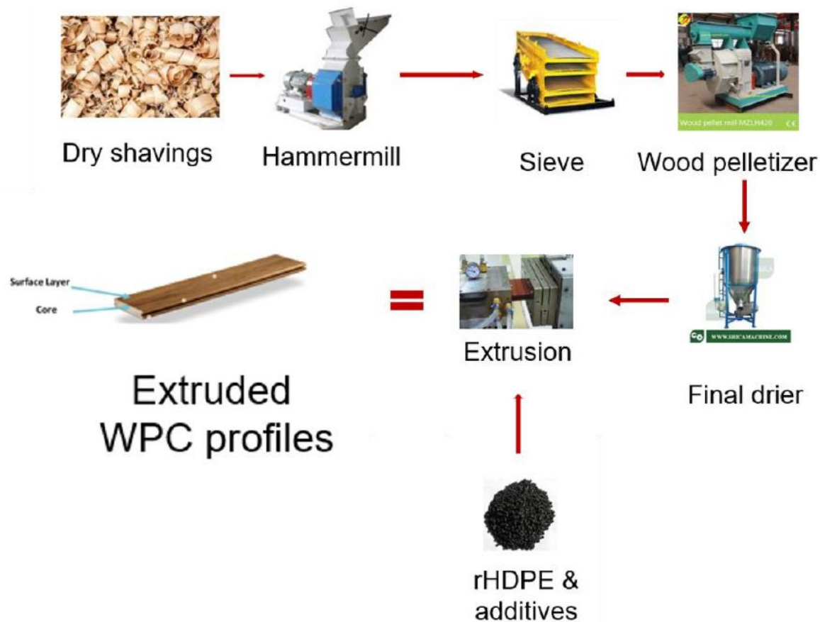
Figure 3-2: WPC Facility process schematic
