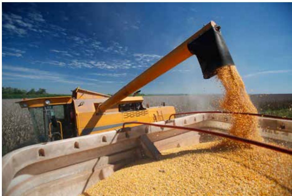
Figure 1: Most harvesters perform best, losing and damaging less grain, when moisture content is >18%.
