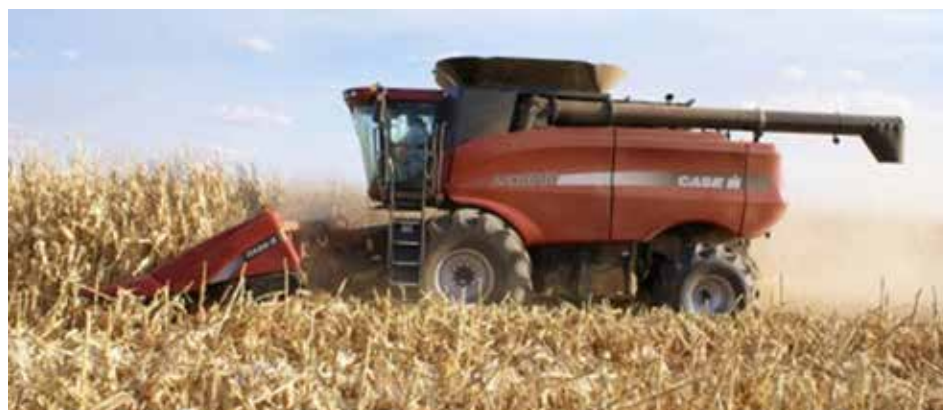
Figure 2: Grain harvesting is normally done with a corn front with either a snapper front or cutter bar (pictured). (Photo: Pacific Seeds)
