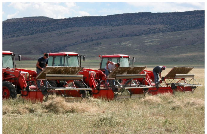
Figure 9. Strippers with hoppers used to mechanically harvest dense small-leaf globemallow stands growing near the Utah-Arizona border. Photo: S. Young, USU.
