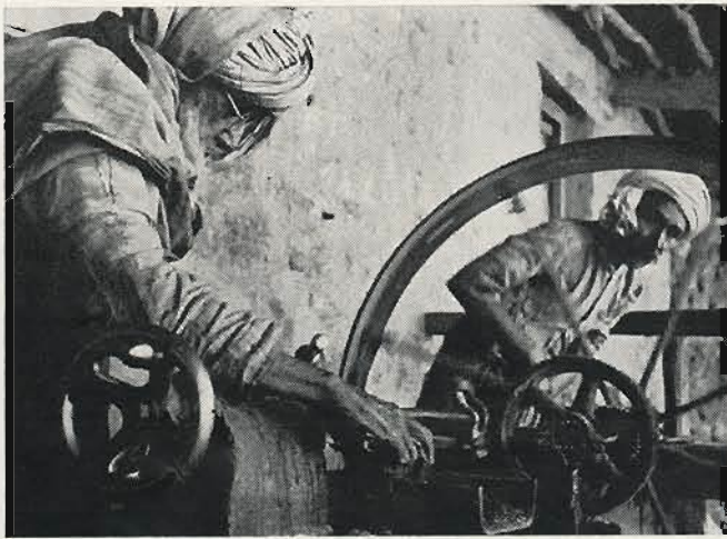
Barrel boring mill is operated by foot power and work is done by eye without help of gauges or other tools.
