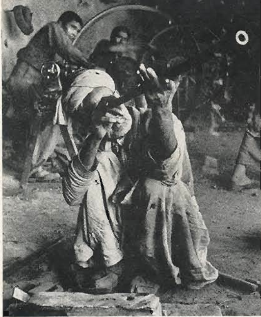
Accuracy of the Darra guns depends largely on skill of barrel straightener's eye and hammer.
