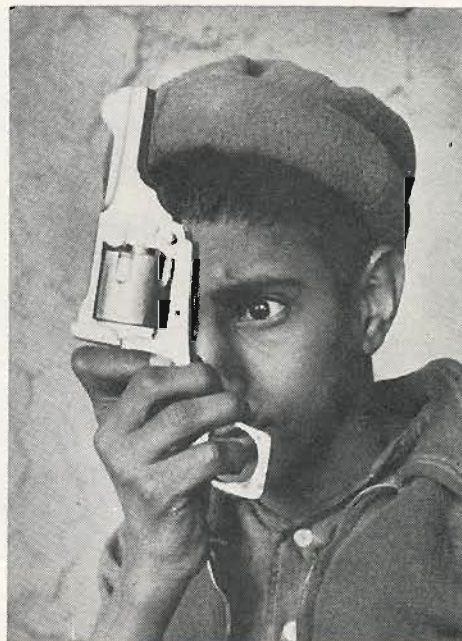
Young tribal gunsmith visually checks headspace of copy of Webley Mark III.
