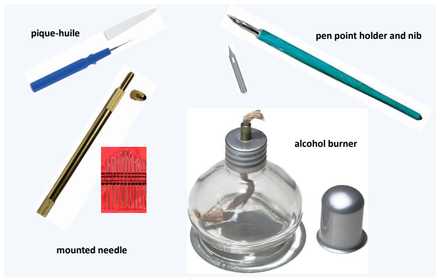
Figure 22 The basic tool kit to work with P. anserina . Pen point holders are used to slice explants of mycelium from jellified growth plates. The ones with replaceable nibs are ideal. Mounted needles or “pique-huile” are used to collect fruiting bodies and ascospores. These tools can be sterilized with an alcohol burner.
