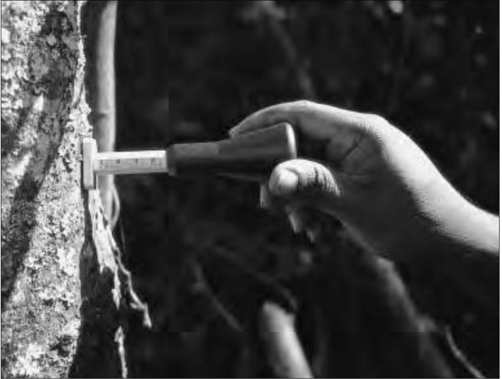
Figure 4.4 A Swedish bark gauge being used to measure the thickness of Prunus africana bark
