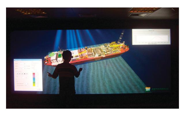
Environ is an application motivated by the need to visualize large industrial engineering models derived from CAD tools. Its main goal is to offer 3D visualization resources with enough realism to be used for virtual prototyping, design review, change-management systems, training, and immersive VR projection facilities.
