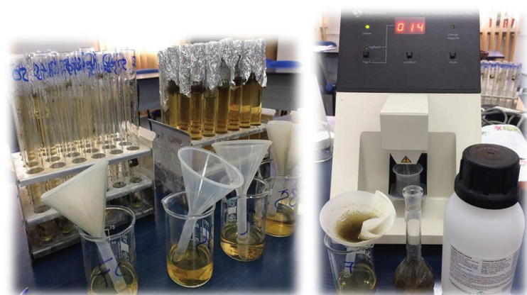
Figure 2. Aspects on how to determine the Cl - content of bean plants with the Analytical Chloride Titrator (original)
