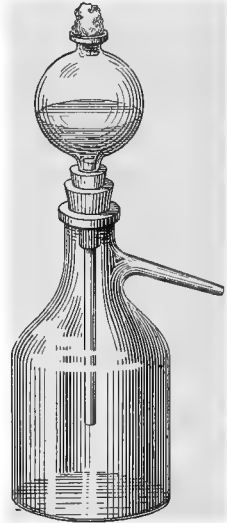
FIG. 33.—Kitasato filter for filtering hypodermic solutions, culture media, sera, water, etc. The material to be filtered is placed in the globose container and forced through the clay (infusorial earth) tube (Berkefeld filter bougie) by connecting the receiver with a vacuum pump. All parts of the filter must, of course, be sterilized by heat before and after using. (Williams.)
