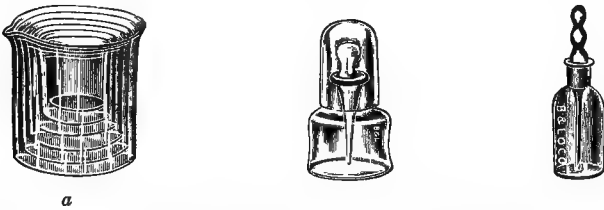
FIG. 11.— a , Nest of beakers and reagent bottles. The smaller and medium size beakers are more desirable for bacteriological work. The reagent bottles are for Canada balsam, stains, clearing fluid, etc.
