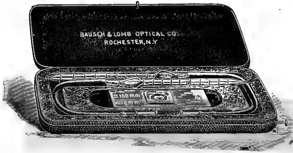
FIG. 39.—Thoma-Zeiss hemacytometer. Complete equipment for blood counting. This is very convenient for making bacterial counts in catsups, jams, jellies and other vegetable foods and also in animal food substances.
