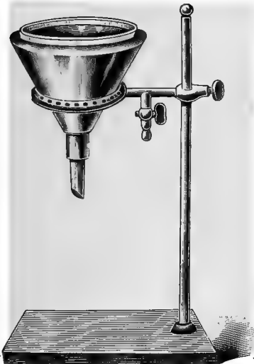
FIG. 26.—Hot water funnel with stand and ring gas burner.
