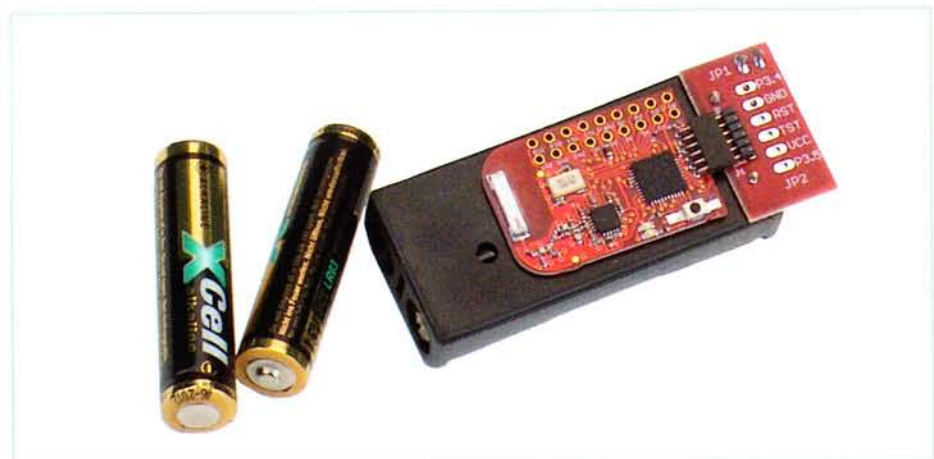
Figure 2. eZ430-RF2500T board used as a remote control module.
