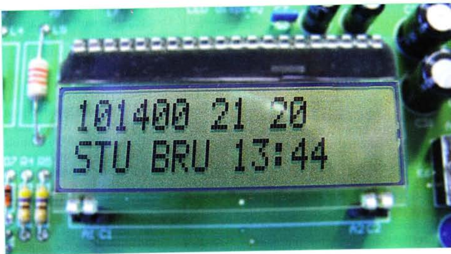
Figure 5. The display shows the currently tuned frequency, the signal strength at the antenna in dB \mu V, and the signal-to-noise ratio (SNR) in dB. When receiving an FM station the lower line of the display shows the RDS station identifier and time of day.
