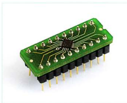
Figure 4. The Si4735 module consists of a daughter board with the DSP IC mounted on it.
