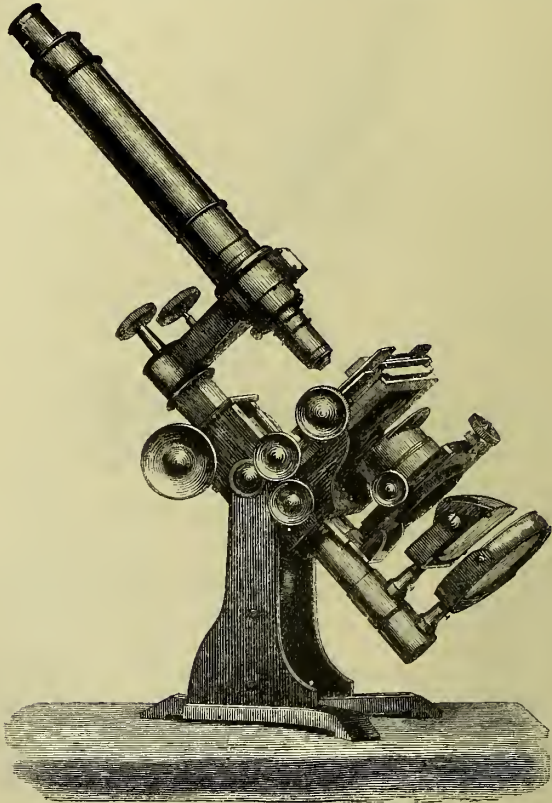
Fig. 42.—Baker's No. 1 Compound Microscope.
