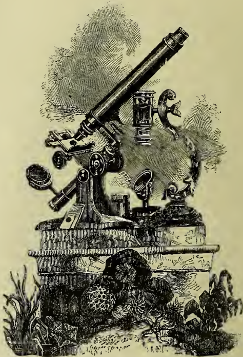
Fig. 3.—Baker's Scroll or Pocket Microscope, and the Modern Compound Microscope of W. Ladd's manufacture.
