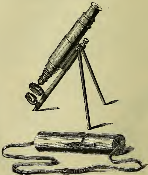
Fig 63.— Baker's Traveller's Microscope.
