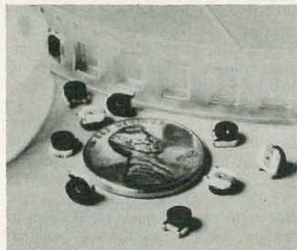
FIG. 8—TRIMMER RESISTORS also come in SMT form; each device is about 4 mm on a side.
