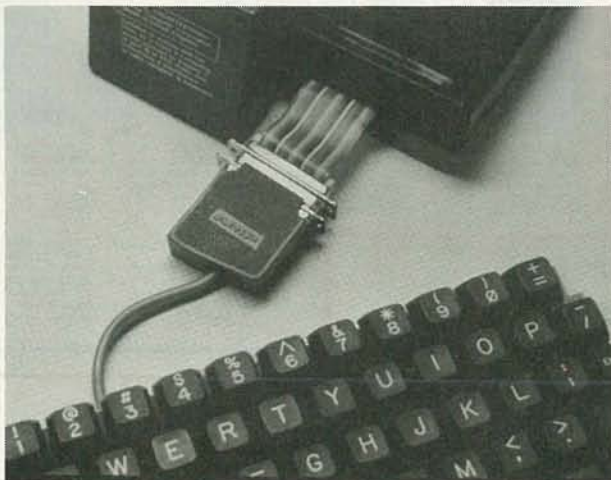
FIG. 5—MALE AND FEMALE DB-25 connectors connect the TI keyboard to the Sinclair motherboard.
