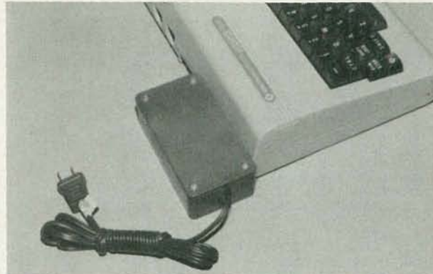
FIG. 11—THIS ILLUSTRATES the power controller connected to the computer. Be sure the connector location is such that the box does not cover the opening for the cassette interface.
