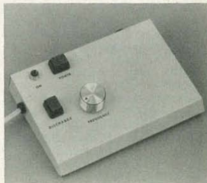
FIG. 5—TO MAKE THEM EASIER TO FIND in the dark, cluster the unit's operating controls around NE1.
