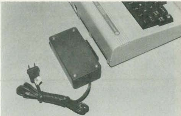
FIG. 10—POWER CONTROLLER plugs into the user port at the rear of the cabinet.
