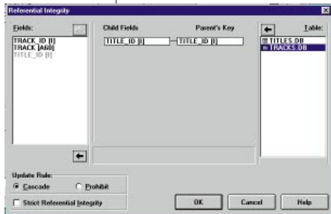
Fig 2 Using the Database Desktop, you can set up referential integrity to prevent orphaned data in your database — for example, tracks with no corresponding title
