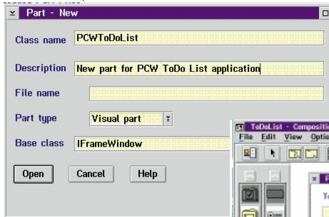
Right In the Composition Editor, the new part is built up by selecting controls from a palette, drawing them in the work area and then editing their attributes
