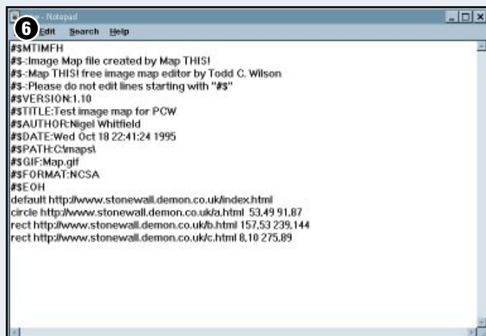
Fig 6 This is the resulting map file, opened with Notepad. All you have to do now is copy it to your Web server
