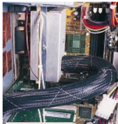
▲ TAKE THE TUBE – THE MAIN ARTERY PUMPING PRECIOUS COOLANT TO THE RACING CPU
