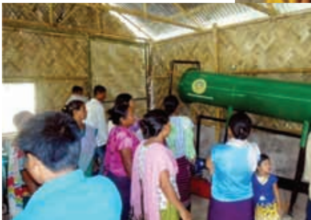
Vacuum pressure impregnation plant
