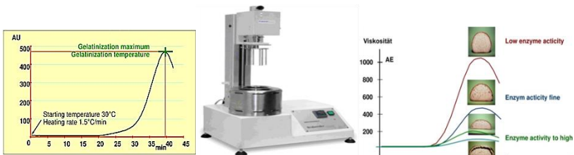
Fig. 11. Amylograph Test Curve (Anonymous, 2012)
