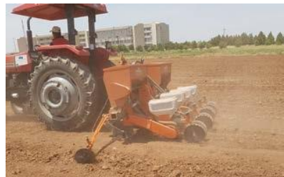
Figure 1. Pneumatic maize drill and combined pneumatic maize drill
