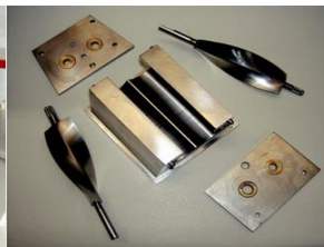
Fig. 20. The Mixolab Dismantled
