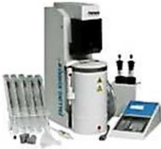
Fig..10. Falling Number Device and Viscosimeter Tubes (Anonymous, 2013)
