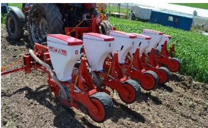
Figure 1. Pneumatic maize drill and combined pneumatic maize drill
