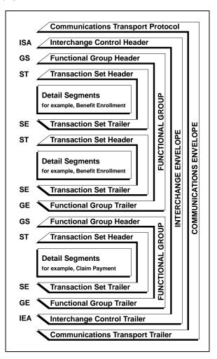
Figure A1. Transmission Control Schematic
