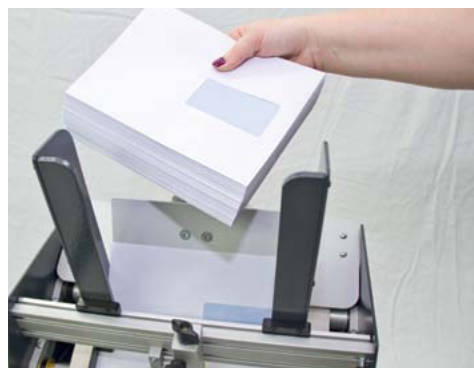
The large capacity Envelope Hopper enables 10 - 1000 envelopes, to be loaded.
