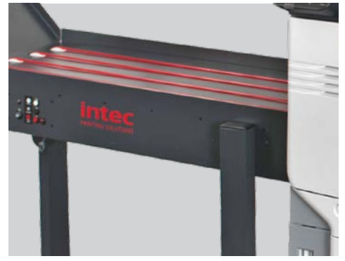
The Shingling Conveyor provides an adjustable/variable overlap of envelopes for quick inspection and easy repacking.
