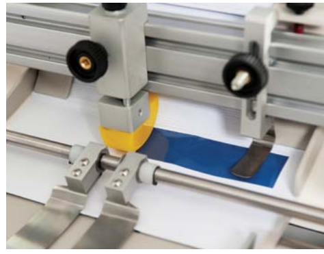
Continuous feed system pulls envelopes from the bottom of the stack, ensuring uninterrupted production as you load from the top.
