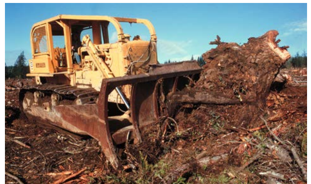
Figure 1: D8 Cat, used to extract stumps in the early days of stumping in western North America.
