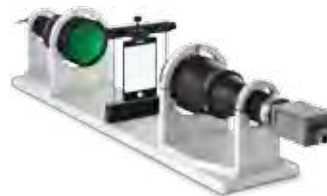
Detection of tiny scratches, bubbles and inclusions on smartphone glass screen.
