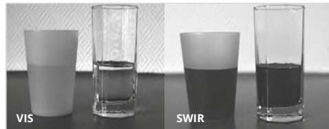
Liquid level inspection
