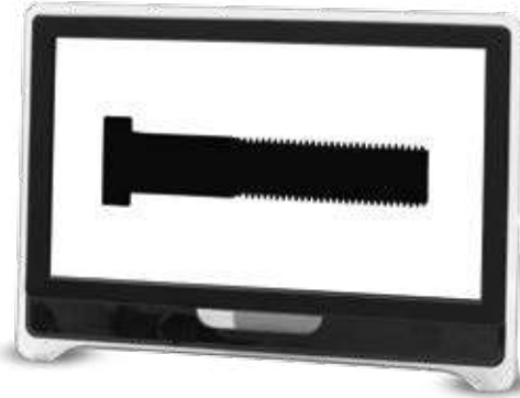
LTCLHP080-x + CMMR080 and TC23080 + CMMR080 imaging a screw in a collimated setup.
