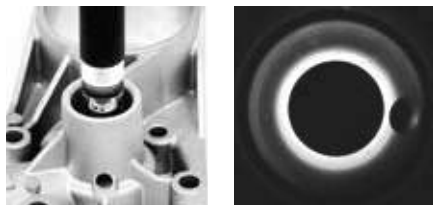
Inspection of holed parts of an engine.
