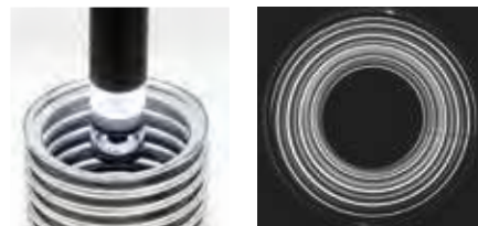
Tube scanning for integrity inspection.
