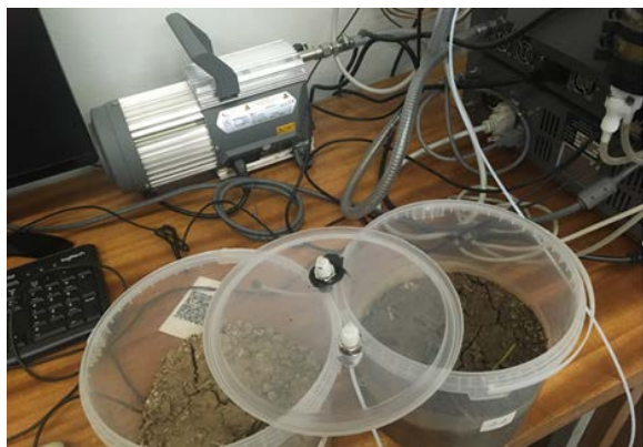
Figure 5. Three liter buckets with mixed soil samples connected with CRDS device Picarro G5131-i.
