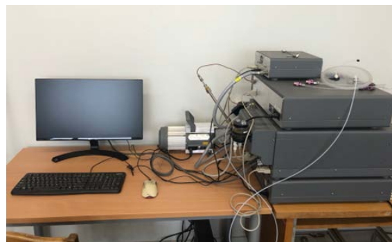
Figure 6. Isotope and gas concentration analyser CRDS device Picarro G5131-i.
