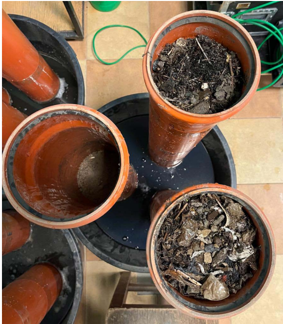
Figure 4. Three experimental tubes. Two with a layer of biocover, one without.
