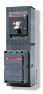
a contactor has breaking capacities at high currents which are less efficient than the circuit-breaker, but a high number of possible operations consistently higher than those of the circuit-breaker (about 1.000.000). The combination of the two devices therefore optimises motor protection and control.
