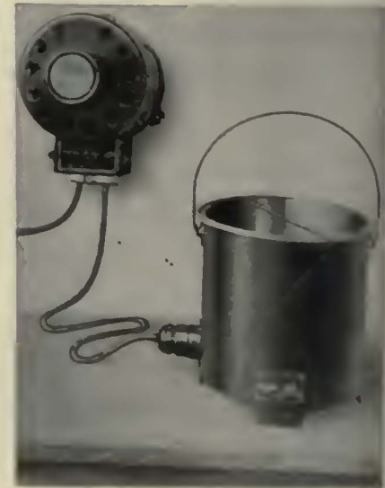
Dry-Type Glue Pot with Rheostat for Heat Control
