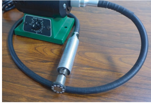
Fig. 1 A specially designed electric tissue roller for high-throughput sample sap preparation
