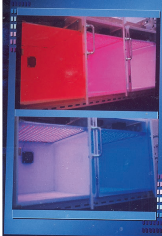
Fig. 2 LED Pack with various blue to red LED ratios
