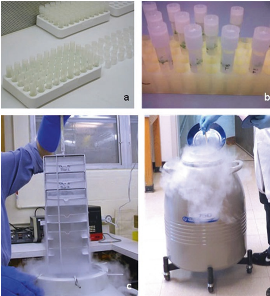
Fig. 4 Cryovials left at room temperature ( 27 \pm 2 °C) prior to the addition of a plant vitrification solution (a, b). Cryovials are placed in racks (c), which are immersed in liquid nitrogen inside a cryotank (d)
