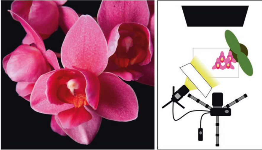
Fig. 3 (a) An example image of a Phalaenopsis flower captured using a professional quality SLR camera (Canon 5D Mk II) and lighting. This image demonstrates the level of quality that can be achieved with a higher complexity and accordingly higher-cost assembly of equipment. (b) As in Fig. 2b, a section of black cloth was placed behind the subject, a white card underneath to reflect light into the shadows and the camera attached to a tripod for stability. A photographic flash unit was used and the light modified by placing a translucent scrim in front of the flash. Not shown is the placement of the subject on a small table leaving room on all sides for the placement of the other equipment
