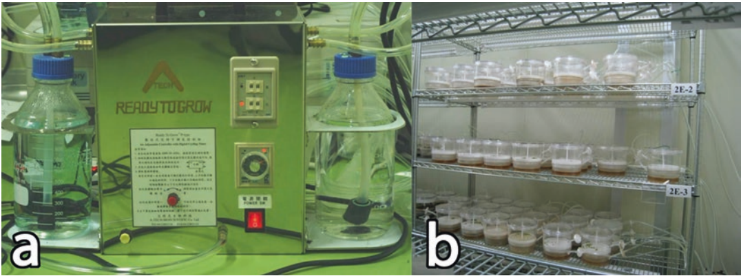
Fig. 6 (a) Basic equipment of the temporary immersion system (TIS) and (b) ventilated Plantima plant tissue culturing containers
