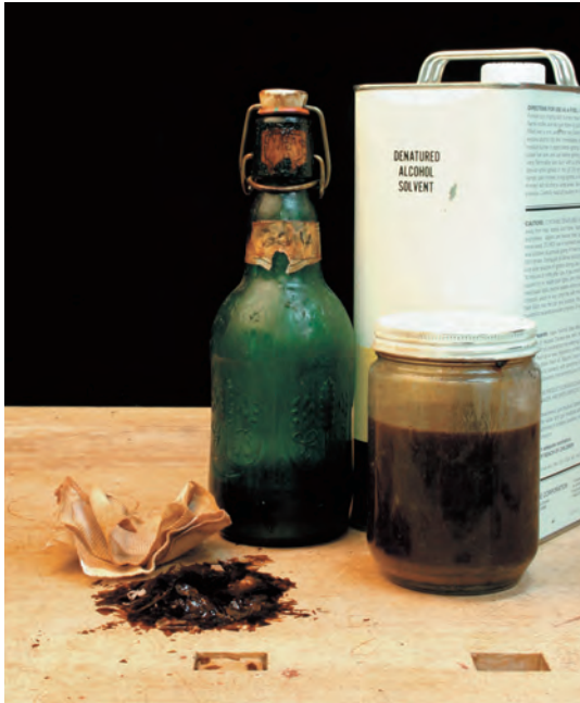
5–42. The products and materials needed for a shellac finish include shellac flakes, a jar of shellac stock solution, an applicator bottle with diluted shellac, grain or denatured alcohol, and an applicator cloth.
