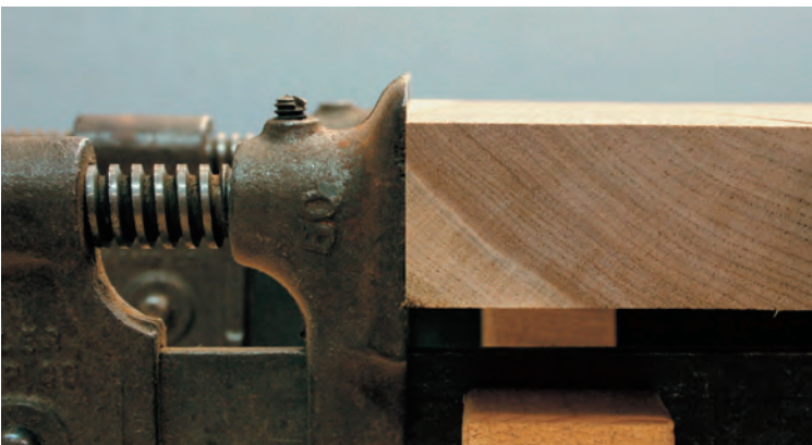
5-22. Aligning the centers of the thickness of the board and the clamp screw minimizes skewing of the joint during glue-up.
