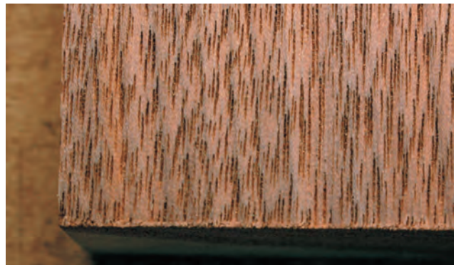
5-35. The scribe line marked on the edge is revealed on the face by planing. Note the fuzzy-looking inner edge.
