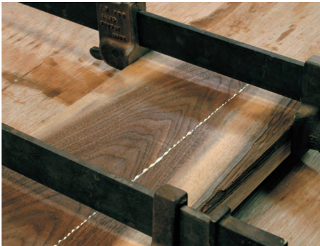
5–25. Squeeze-out as seen from underneath the board. It is a little heavier than need be.
