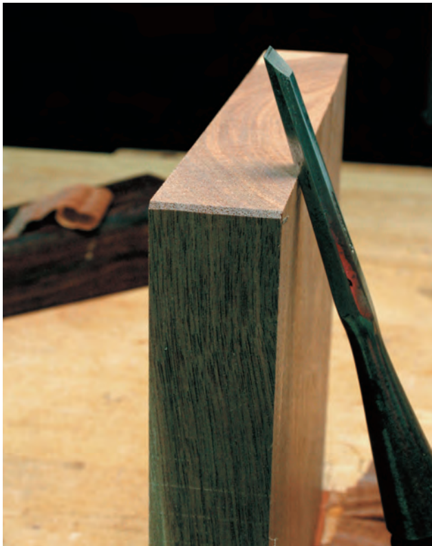
5-38. Chamfering the corner of the board.
