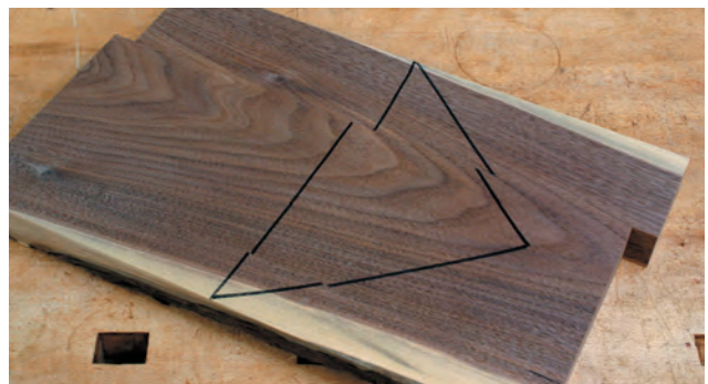
5-14. Saw cuts in straight and angled grain areas of a board. Notice the degree of offset at the ends of the boards required to match the grain when the cut is made in an area with angled grain lines.
