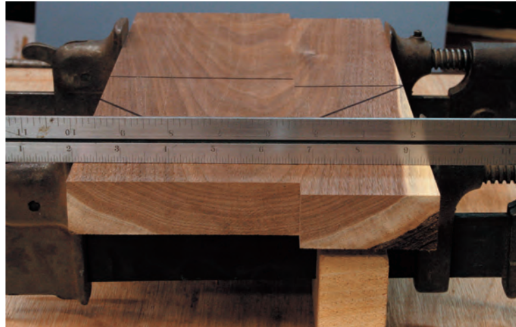
5–24. Checking for flatness across the boards with a straightedge.
