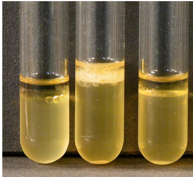
A. B. C. Figure 2: Emulsification of diesel oil by bacteria A. and C.: Top layer of non-emulsified diesel B.: Emulsified diesel can be seen on aqueous layer of bacterial culture.
