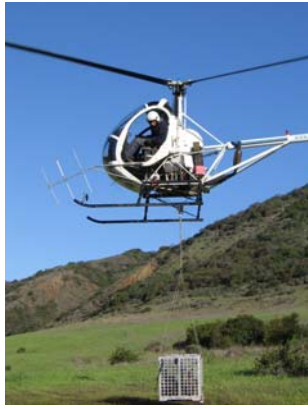
Deploying Judas animals and radio telemetry collars in use at Santa Cruz Island, California. Note the multi-frequency, specially modified antenna in use on the helicopter used for tracking.
