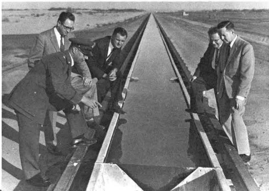
Here is the windup end of the nearly four-mile-long supersonic sled track at Edwards AFB. If it looks like water, it is . . . the last 6,000 feet of it to provide braking. That's Lt. Col. Earl R. Strandberg in uniform. Kodakers, from left, are Walt Fallon, Bob Buchanan, Walt Litten and Don Kridel.
