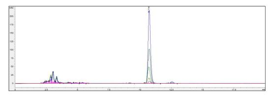
**Figure 3.** LC-UV-chromatogram of ergosterol obtained with chloroform-methanol extraction from the marine fungal isolate *Rhodotorula sphaerocarpa*. Five fungal dilutions in artificial seawater are shown ( $4 \times$ ,  $8 \times$ ,  $16 \times$ ,  $32 \times$ , and  $64 \times$ ), and the *x*-axis shows minutes of the run.
