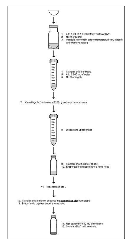
Figure 7. Ergosterol extraction method modified and adapted for pelagic fungi.
