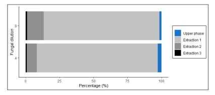
**Figure 1.** Percentages of ergosterol extracted with chloroform-methanol approach from two fungal dilutions ( $4\times$ , and  $8\times$ ) of the marine fungal isolate *Rhodotorula sphaerocarpa*. Extracts recovered from the upper (one extraction) and lower (three extractions) phases were analyzed.
