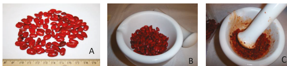
Figure 5. Study material. A: Seeds were separated from mature fruits; B: seeds were prepared and gently crushed in a mortar and pestle (C), and were subsequently hydrodistilled. Photos courtesy of V.R and N.T.
