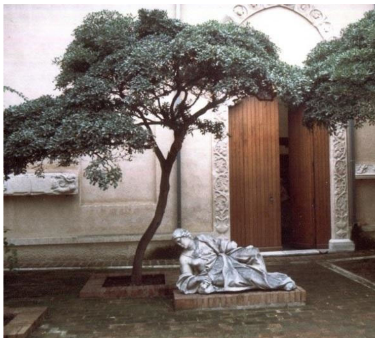
Figure 4. Extended black-greyish patina due to black fungi colonization on marble statue located in the inner yard of the Museum of Messina, Italy, under a tree of Pittosporum tobira . Fungal strains isolated from the statue were attributed to meristematic black fungi and genera of Cladosporium , Alternaria and Phoma Ref. [81].
