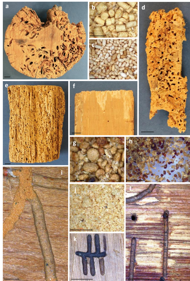
Figure 3. Galleries, exit holes, and dust excrements of several widespread wood-deteriorating beetles in Europe. (a) Cross-section of a utility pole with oval galleries bored by Hylotrupes bajulus (Cerambycidae). Note that galleries are present in sapwood only. Bar = 10 mm. (b) Cylindrical dust excrements characteristic of Cerambycidae. Bar = 1 mm. (c) Dust excrements of Anobium punctatum (Anobiidae). Bar = 1 mm. (d) Piece of a wooden pillar attacked by members of Curculioninae (Curculionidae). Bar = 10 mm. (e) Piece of wood heavily attacked by members of Anobiidae. Bar = 10 mm. (f) Piece of a skirting board attacked by members of Lyctinae (Bostrichidae). Note the presence of longitudinal galleries covered by dust. Bar = 10 mm. (g) Dust excrements of Xestobium rufovillosum (Anobiidae). Bar = 1 mm. (h) Dust excrements characteristic of Curculioninae (Curculionidae). Bar = 500 \mu m. (i) Detail of a larval gallery bored by members of Lyctinae (Bostrichidae) and partially filled with dust excrements, which are soft to the touch. Bar = 2 mm. (j) Detail of the amorphous dust excrements characteristic of Lyctinae (Bostrichidae). Bar = 1 mm. (k,l) Galleries and exit holes bored by members of Scolytinae (Curculionidae). Note the dark staining of the galleries as a consequence of the growth of ambrosia fungi. Bar = 10 mm.
