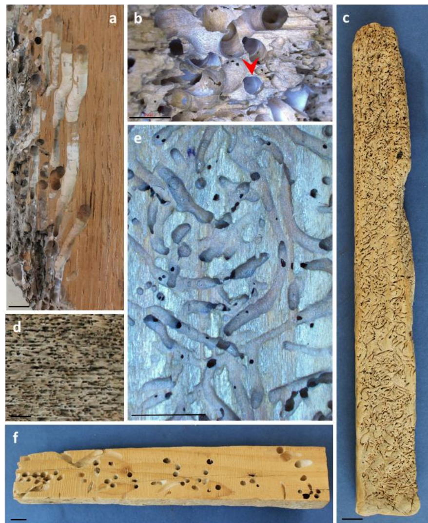
Figure 6. Galleries bored by marine wood borers. (a) Tangential cut of a wooden piece showing internal galleries bored by marine molluscs known as ‘shipworms’ (Teredinidae). Note that galleries follow the fibre direction and are covered by a calcareous lining. Bar = 10 mm. (b) Detail of the galleries bored by shipworms showing the calcareous layer deposited by the mollusc in the galleries (arrowhead). Bar = 5 mm. (c) Wooden piece attacked by crustaceans known as ‘gribbles’ (Limnoriidae) and eroded by weathering, leaving internal galleries visible. Note that galleries are superficial and follow any direction. Bar = 10 mm. (d) Detail of the exit holes of gribbles in wood. Bar = 10 mm. (e) Detail of the tunnels bored by gribbles. Bar = 5 mm. (f) External aspect of a wood attacked by shipworms showing entrance holes. Bar = 10 mm.
