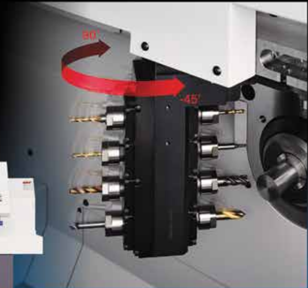
Rotary tools on the gang tool post feature B axis control (Type XII)
