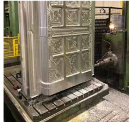
Roughing a cavity plate of a mould and removing aluminum from the block to achieve the general shape before finishing the process.
