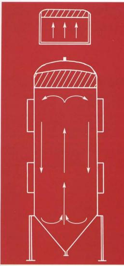
Fig. 2. Comparison of a traditional open rectangular vessel and a modern cylindro-conical fermentation vessel, drawn to the same scale. The shaded section represents head or froth above the fermenting beer; the arrows show the direction of currents within the fermenter.
