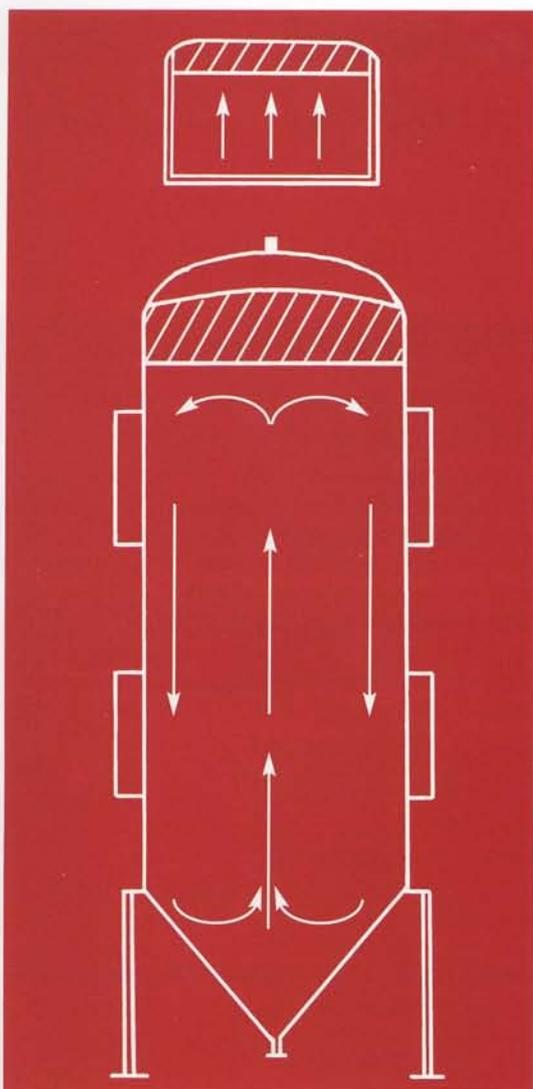
**Fig. 2.** Comparison of a traditional open rectangular vessel and a modern cylindro-conical fermentation vessel, drawn to the same scale. The shaded section represents head or froth above the fermenting beer; the arrows show the direction of currents within the fermenter.
