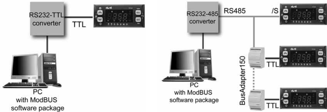
ModBus - Connection diagram of single controller via TTL
