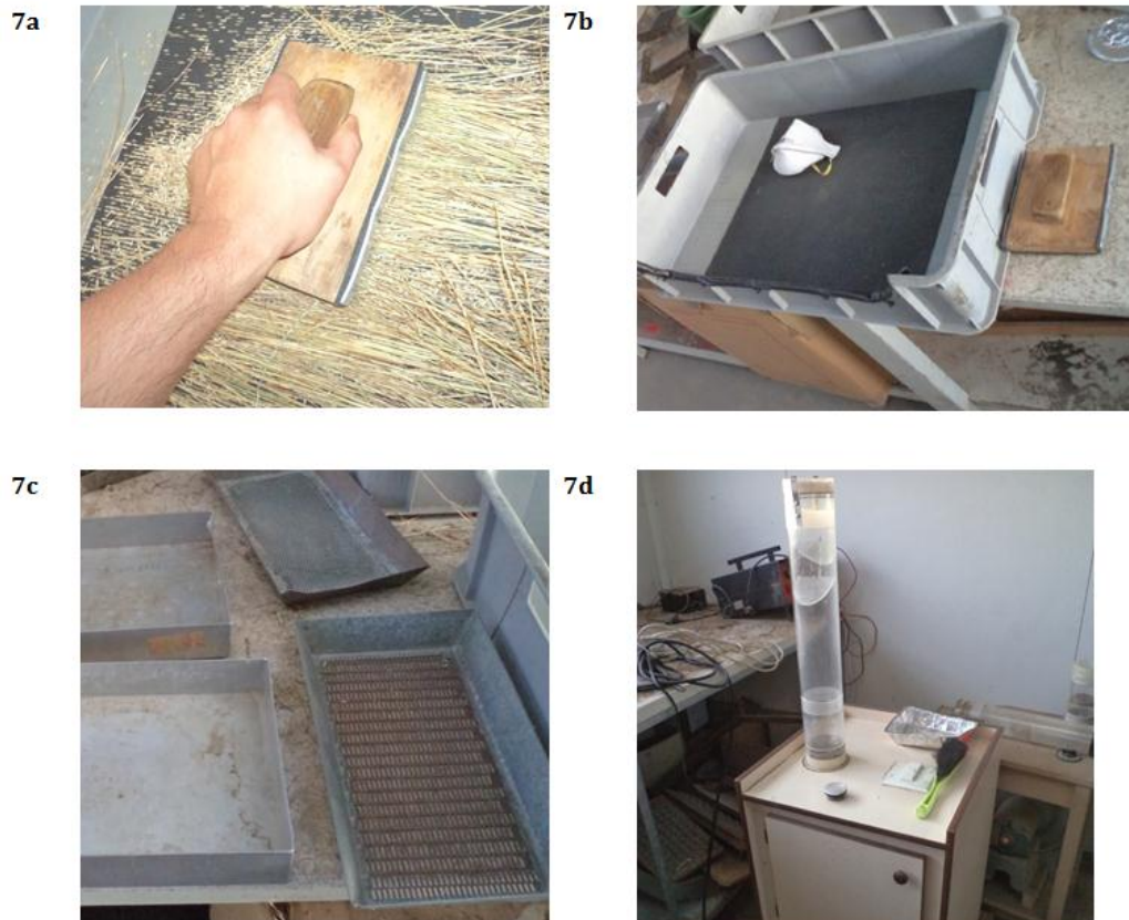
Figure 7: (a) Hand rubbing; (b) Plastic container; (c) Metal sieves; (d) South Dakota seed blower.
