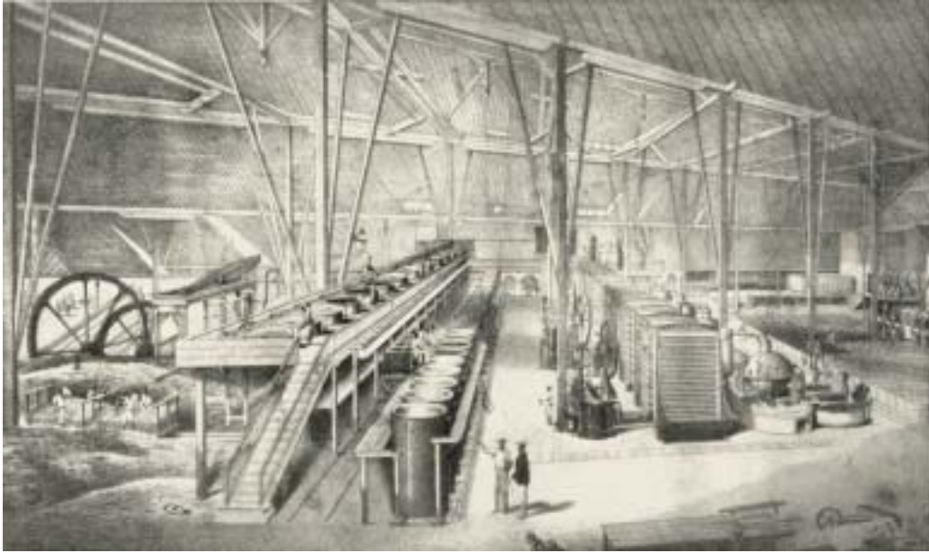
Figure 3.13. Inside a Nineteenth-Century Sugarhouse. The wheels of the mill are seen to the far left. The rows of boiling kettles in the center are an elaboration of the Jamaican train. The filtering cisterns and vacuum pans for final crystallization are to the right. From Geoffrey Fairrie, sugar (Liverpool, 1925), Plate 59, opposite page 158.
