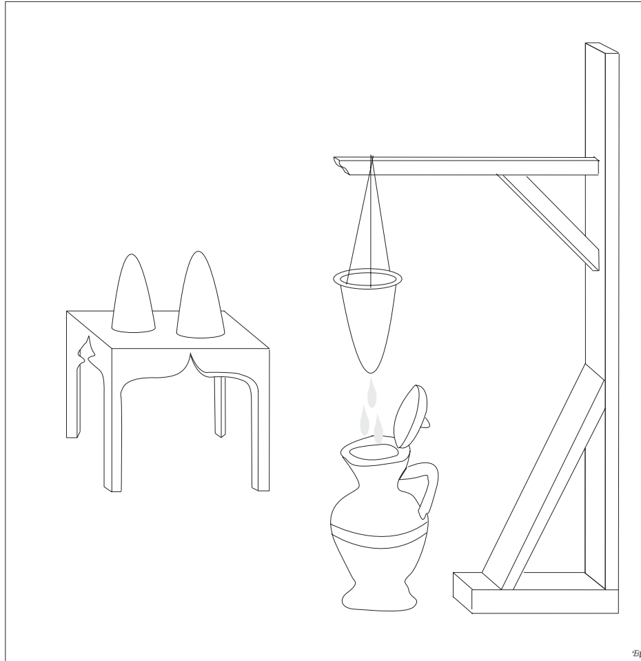
Figure 3.14. Fifteenth-Century Venetian Draining Cone and Sugar Loaves. The massecuite was placed in a cone-shaped mold and the draining molasses was collected in a vessel positioned below the mold. The resulting sugar "loaves" are shown on the adjacent table. Drawn from a photograph in Fernand Braudel, Civilization and Capitalism 15th-18th Century . Vol. 1 (New York, 1992), 225.
