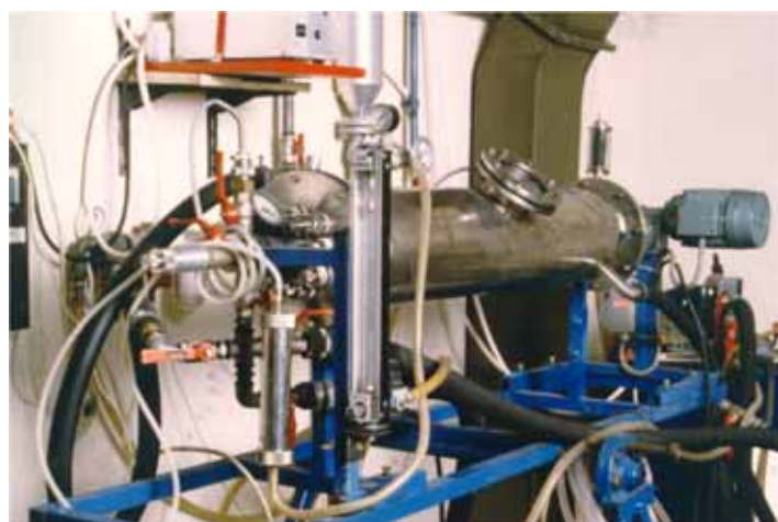
Figure 1. Horizontal stirred tank reactor and equipment
