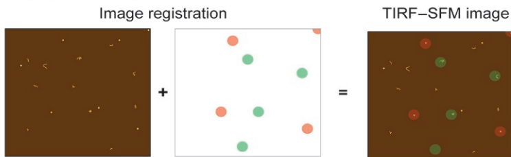
Fig. 8 Overview of steps in experiments applying TIRF-SFM imaging. Schematic representation of sample preparation steps, image collection aspects, and required post collection image processing to create merged fluorescent and topographic data.
