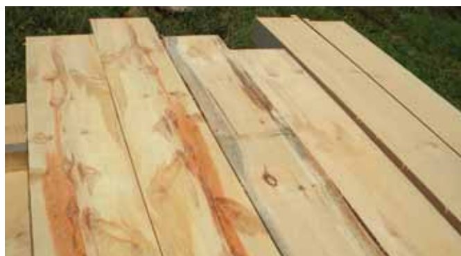
The reddish stain on the two boards at left is red rot.
