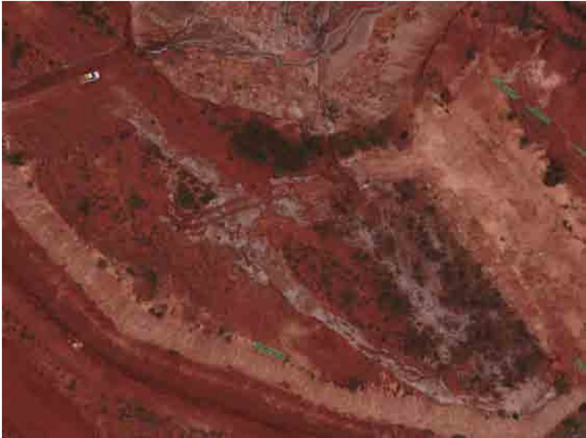
Figure 12 - Aerial view showing extent of saline crust left behind once hypersaline spill had evaporated
