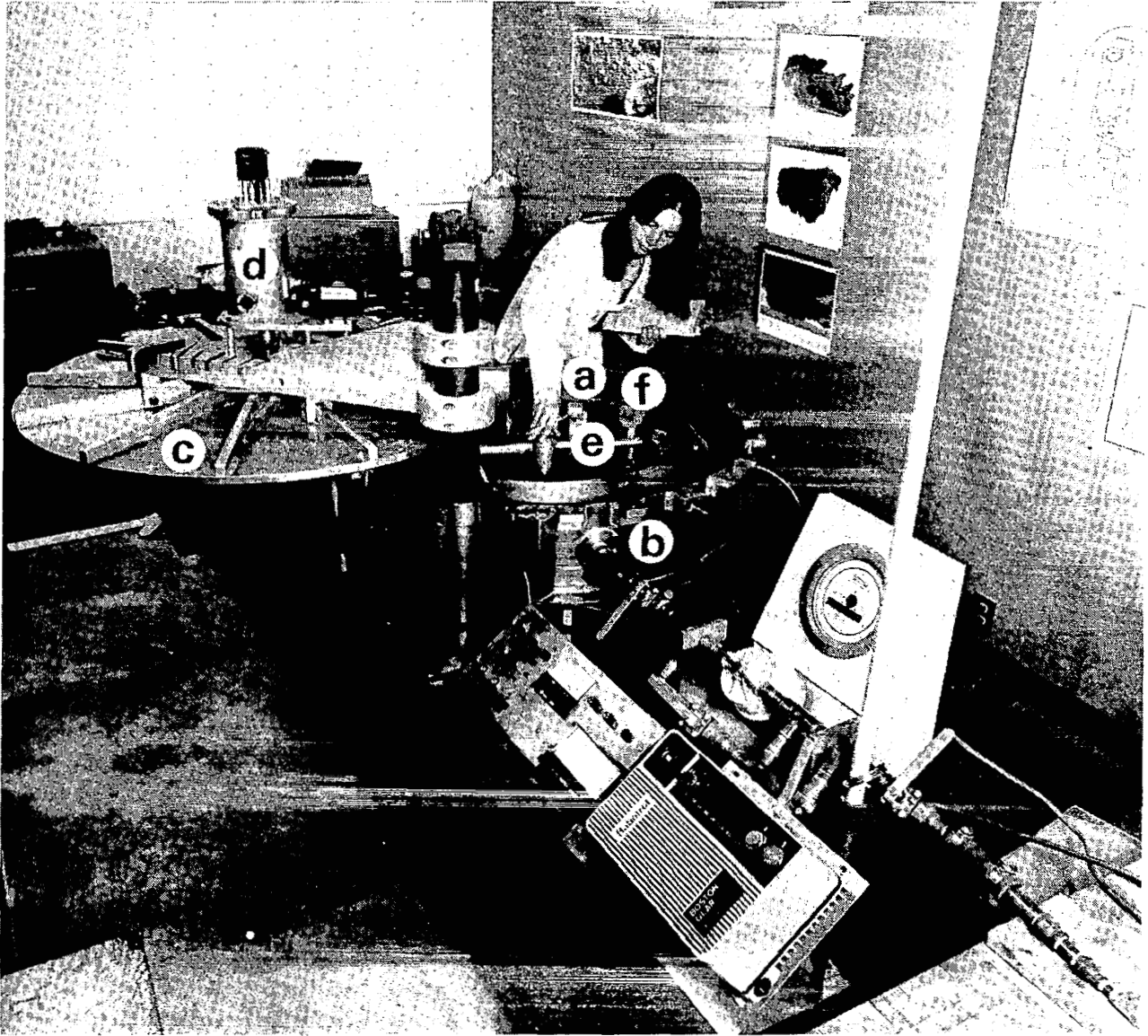
Figure 29. View of the apparatus used to conduct experiments to determine susceptibilities to erosion ( S_a ). Samples to be abraded are placed in holders (a) positioned within cylindrical chamber (b); cover for chamber (c) swings into position such that abrading particles (quartz sand, etc.) in hopper (d) are fed into rotating arm (e) where they are slung against the samples; speed of arm controls the impact velocity; sample holders (a) can be adjusted to control impact angle; 12 samples can be abraded per experiment; one sample station (f) is modified as an open port to collect the same amount of material as strikes each sample to enable an accurate determination of particle flux. Control panel is shown in foreground; chamber can be evacuated to low atmospheric densities and carbon dioxide can be introduced for martian simulations (from Greeley et al., 1982).
