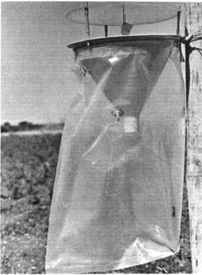
A funnel and bag pheromone trap, used for monitoring H. armigera male moths in collaborative investigations with the Tropical Products Institute, and the Centre for Overseas Pest Research, London, being tested in an ICRISAT field. The trap was designed by Dr. D. Champion of COPR.
