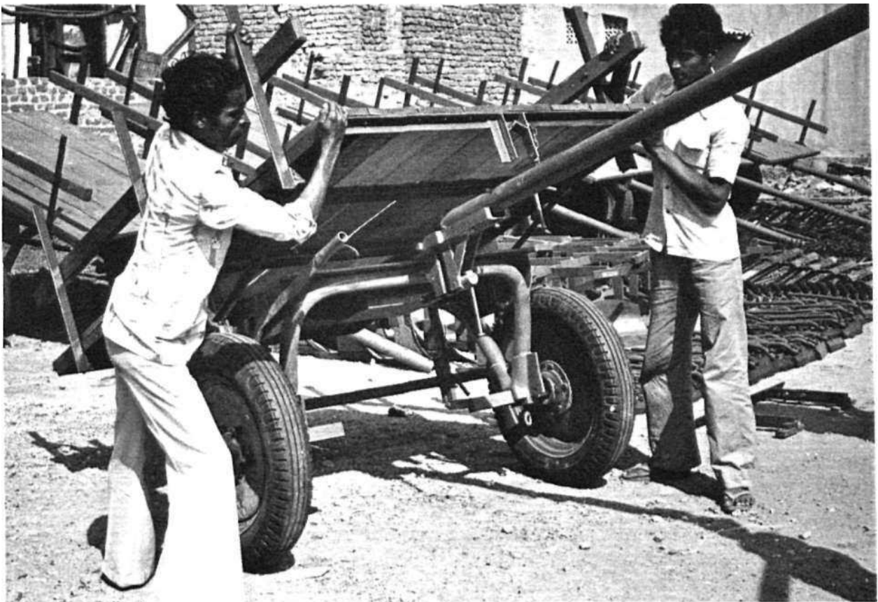
The wheeled tool carrier converted into a transport cart at a manufacturer's outlet in Hyderabad, India. ICRISAT's technical support to manufacturers of improved farm equipment enables better access to such equipment for farmers.
