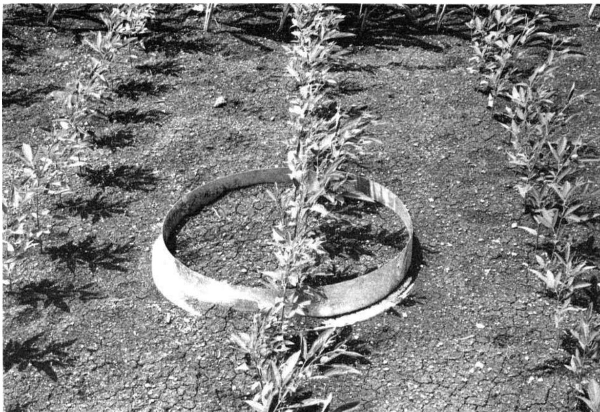
Studying nitrogen fixation: 35-day old pigeonpea plants seen growing within and outside a cement cylinder filled with soil that had been labeled with ^{15}\text{N} fertilizer. A metal sheet helped raise the cylinder rim above ground level to prevent mixing of unlabeled soil from outside.
