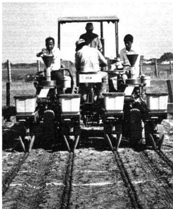
Figure 1. Mechanized planting at a uniform depth of 5 cm with a cone planter on a Vertisol, ICRISAT Center, 1983.
