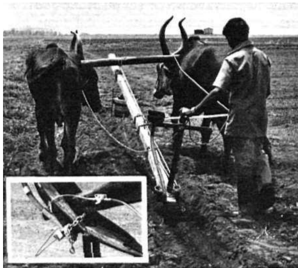
Applying inoculum as liquid to the soil below seeds with a bullock-drawn seeder: this method has proved more effective than conventional methods of inoculating groundnut seeds with Rhizobium strains. Inset shows inoculum flowing into the seeder.
