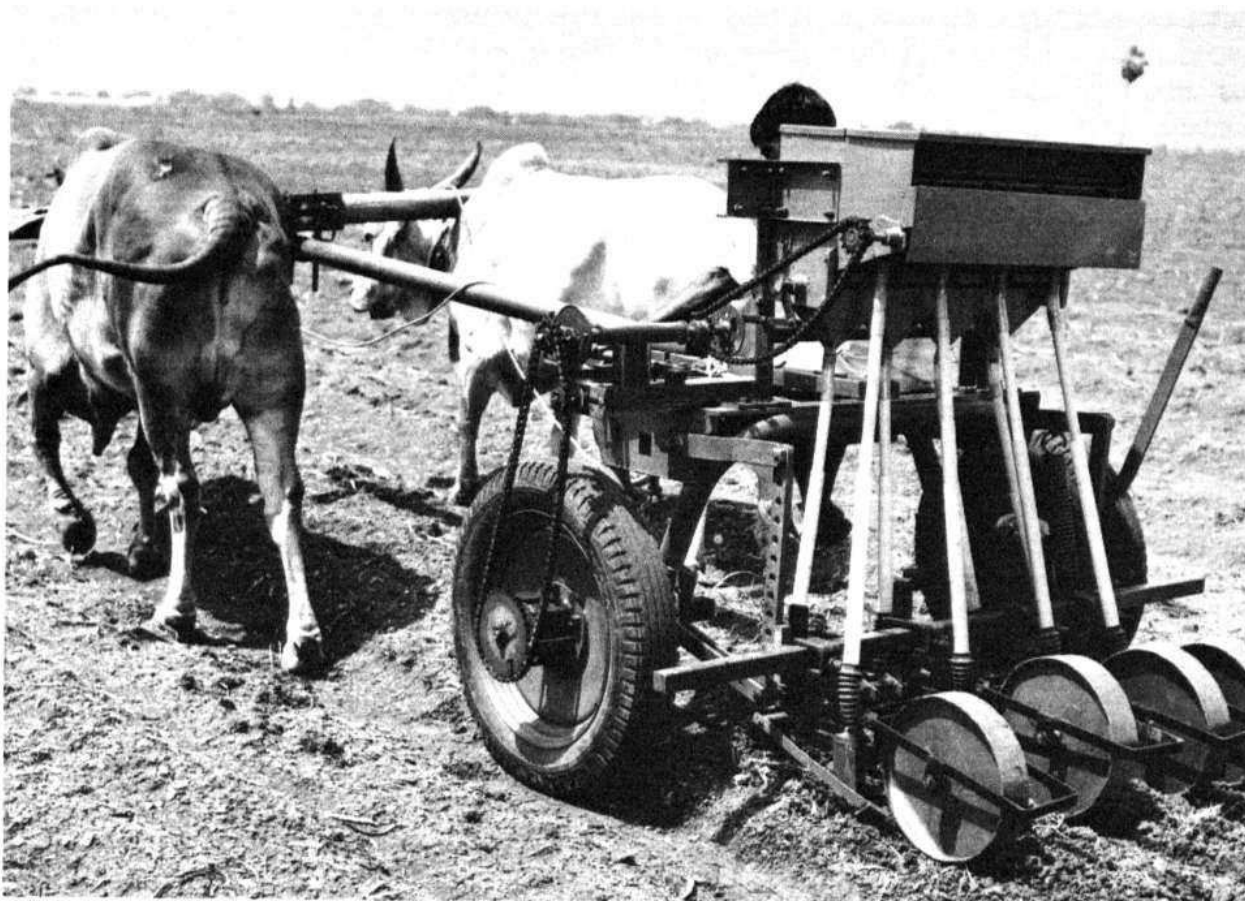
This planter, developed by ICRISAT, meters both seed and fertilizer and places them at the desired depth in the soil, for up to 4 rows in a single pass. It is readily attachable to the wheeled tool carrier, as shown above.
