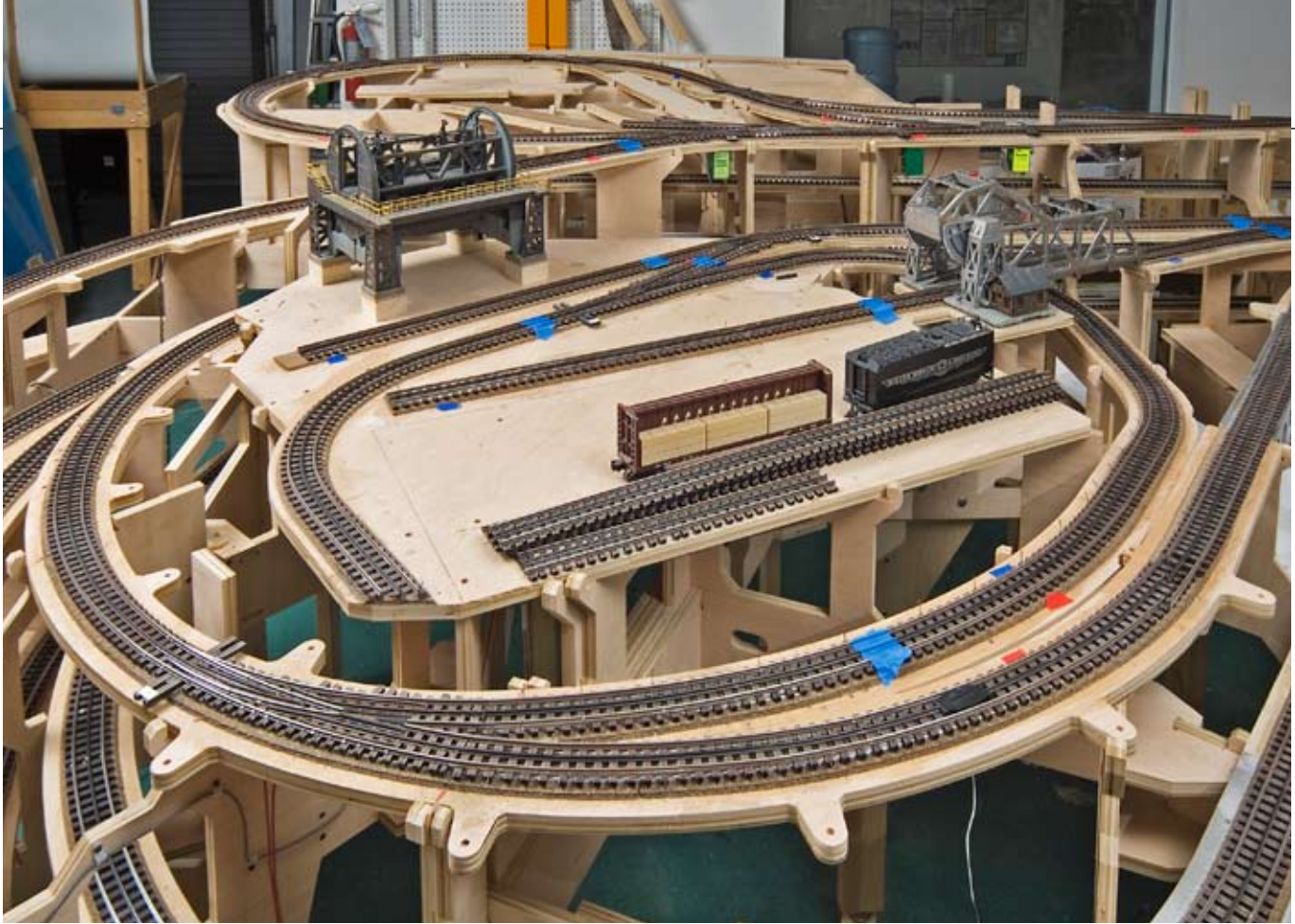
▲ The plywood “puzzle pieces” for the modules on this O gauge layout are cut out by a computer-controlled router before being assembled to form the benchwork and subroadbed. The finished pieces fit together precisely. Now GarGraves flex-track and Ross Custom Switches turnouts, plus a few Lionel accessories, are being installed. In the foreground you can also see where custom-made catenary poles will be erected along the main lines.
