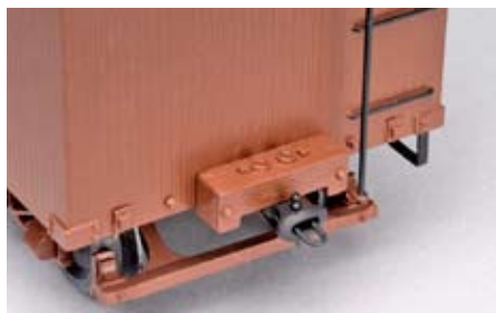
Here is the boxcar's coupler pocket with a link and pin installed.
